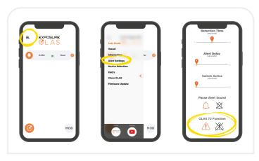
**4.** If using an OLAS T2 go to 'Alert Settings' in the menu and select the alert function for the OLAS T2. Now when you switch off your OLAS T2 tag it will activate the alarm immediately.
