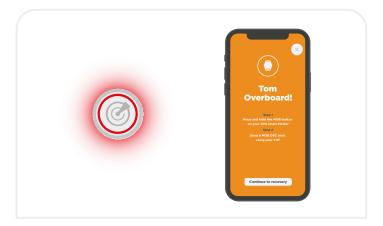
**5.** The alarm will occur after your set 'Alert Time' and the engine will cut out. The default Alert Time is 2 seconds.
