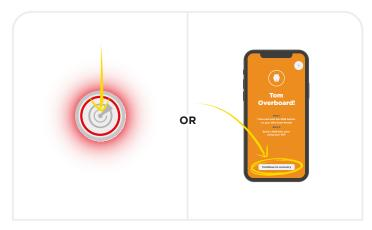
**6.** Press the Guardian's control switch once or tap "Continue to Recovery" in the App. This puts the system into pause state.
