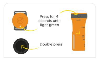
8. Switch the OLAS transmitter back ON.
