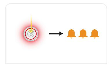
**7.** Press the control switch again once. 3 beeps will sound to indicate that the transmitter is still missing, and the system is still in pause state.
