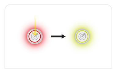
**10.** Press the control switch once, the system will be operating again. Solid green on the control switch indicates it is tracking correctly.
